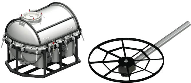
SPIDER FOR MOUNTING MULTIPLE MOULDS ON A STRAIGHT ARM
